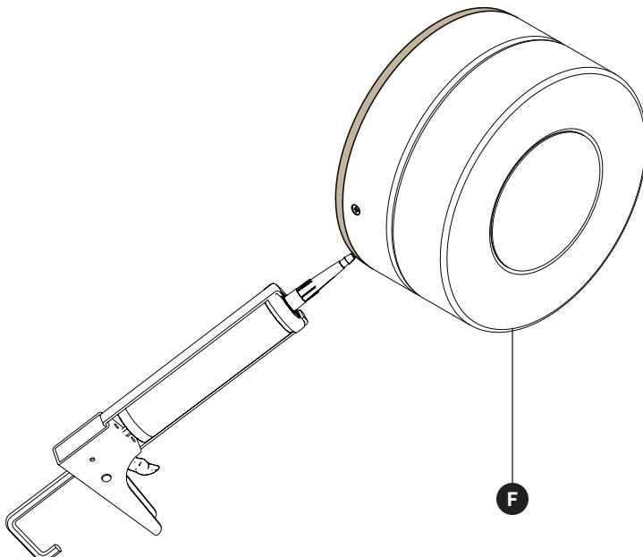
**NOTE:** We recommend keeping the bottom unsealed. To maintain a drainage area in case of water infiltration.
